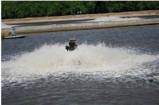
*Typical mechanical surface aerator at work. It is often difficult for this type of machine to aerate the entire water column.*
