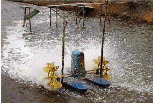
*A one-horsepower paddlewheel aerator. The splashing may increase the evaporation rate of the water and thus increase the salinity of the water body.*
