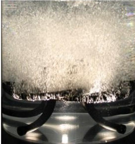
*Fine bubble aeration is an efficient technique of aeration in terms of oxygen transfer due to the large collective surface area of its bubbles.*
